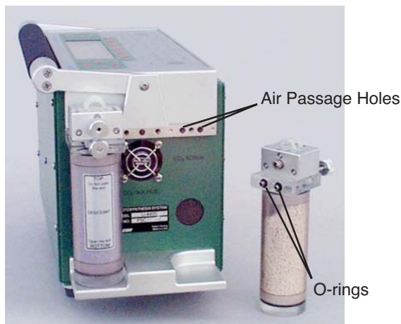
Figure 19-3. Each chemical tube has two air passage holes protected by O-rings.
