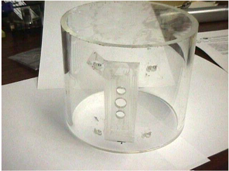
Figure 16-75. A section of Plexiglas tube to be used as a chamber.
