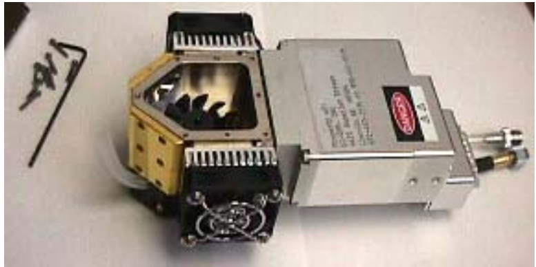
Figure 16-72. The LI-6400 sensor head, leaf chamber removed.
