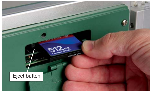
Figure 10-15. Inserting a Compact Flash card into the expansion slot.
