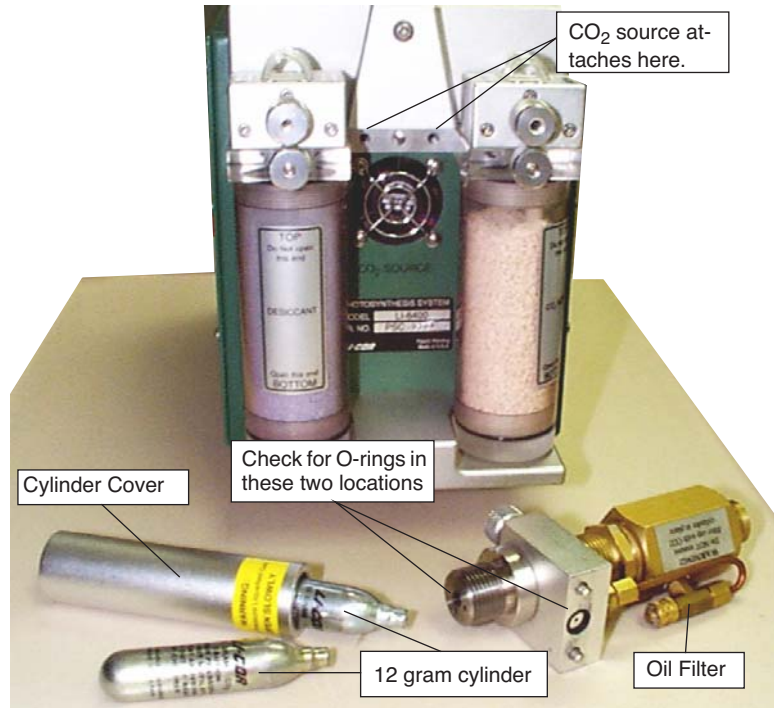
Figure 2-6. Location of external CO 2 source assembly.
