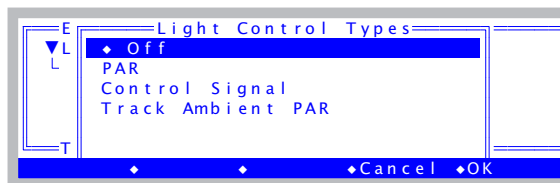
Figure 16-35. Default light settings. The dialog will be the one associated with whatever the light source is specified to be.
