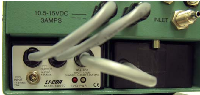
Figure 2-14. The 6400-70 AC Module fits in a battery compartment in the console. If you install a battery in the other compartment, and plug it into the module (as shown here), that battery will trickle charge, but more importantly, provide continued operation for 1-2 hours in the event of a mains power failure.
