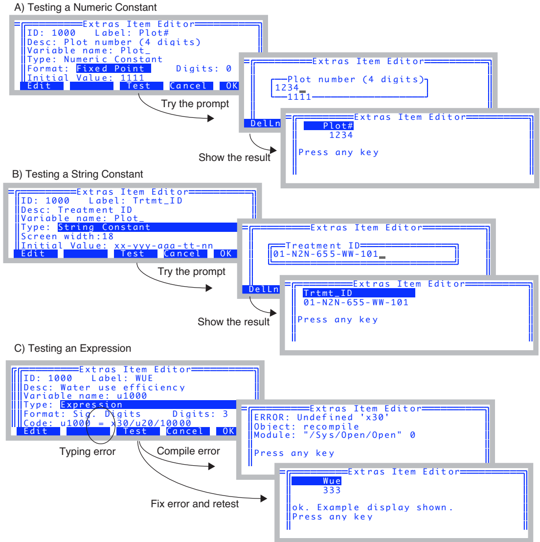
Figure 15-8. Testing A) a numeric constant, using the specified format, digits, description, and initial value; B) a string constant, using screen width of 18; C) an expression, with a typing error so it won't compile.
