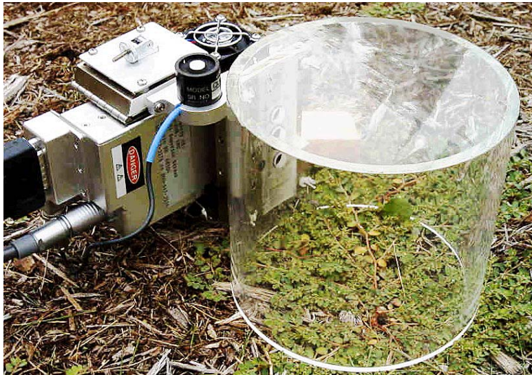
Figure 16-80. Plexiglas chamber measuring Prostrate Spurge
