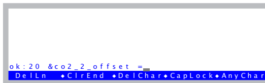
Figure 3-49. Forcing a 20 ppm mismatch in the IRGAs.
