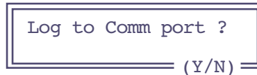
Figure 9-4. The alternate destination prompt. Press Y for Comm port, or escape to cancel logging.
