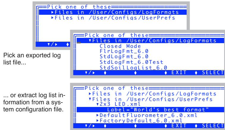
Figure 9-16. Importing a log format. It can come from an exported list, or be extracted from another system configuration file.
